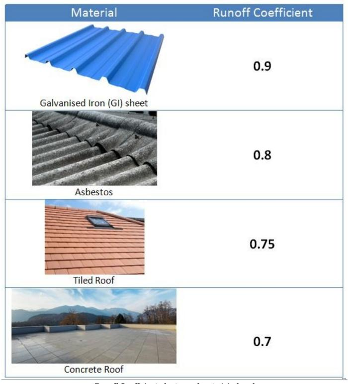
Runoff Coefficients for type of material of roof
