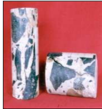
Photo 10- Core after grouting
